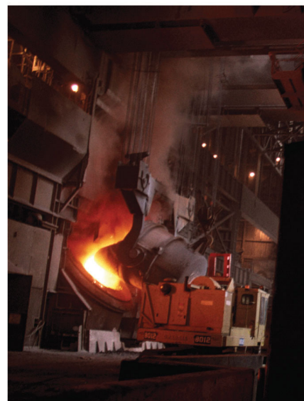
(b) Oxygen furnace in Ohio steel mill
