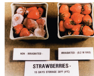
Figure 20.24 The Preservation of Strawberries with Ionizing Radiation
