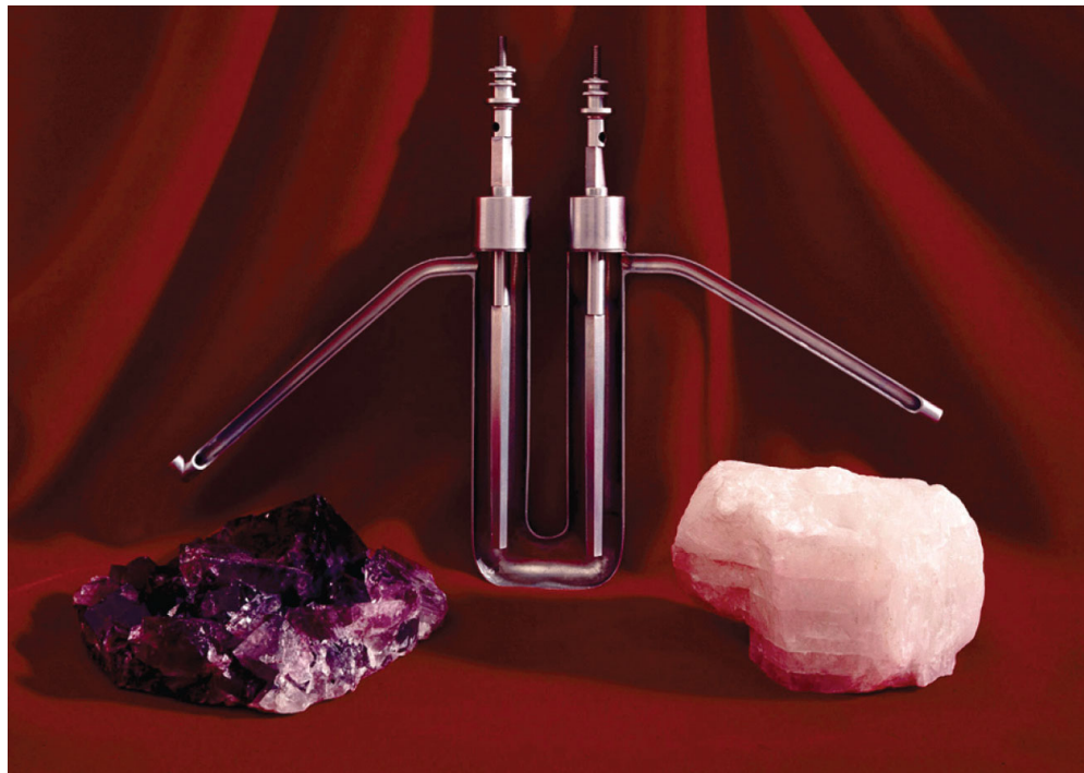
Figure 22.14 Isolation of Elemental Fluorine
