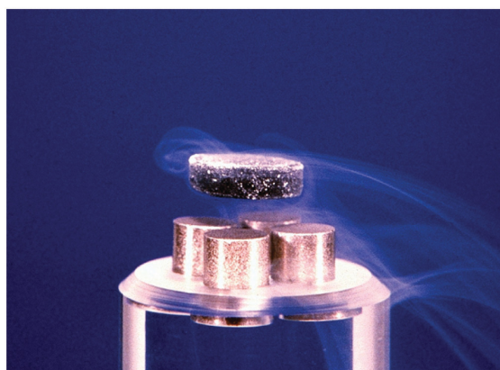
(a) Below its T_c , a superconductor completely expels magnetic lines of force from its interior. (b) In magnetic levitation, a small magnet “floats” over a disk of a high-temperature superconducting material ( \text{YBa}_2\text{Cu}_3\text{O}_{7-x} ) cooled in liquid nitrogen.
