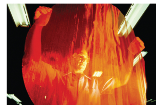
A heterogeneous catalyst. This large circular gauze, woven from rhodium-platinum wire, is a heterogeneous catalyst in the commercial production of nitric acid by the oxidation of ammonia.
