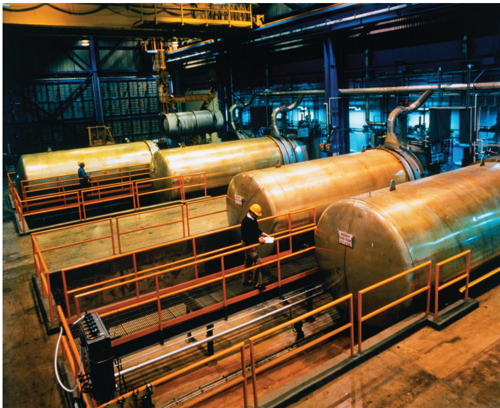
Figure 10.18 A Portion of a Plant for Separating Uranium Isotopes by Effusion of \text{UF}_6
