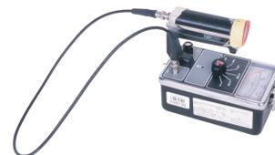
A Geiger counter is a common instrument used to detect radioactivity.
