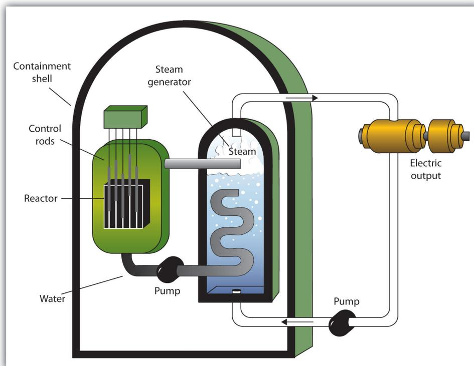
The two main components of the power plant are the nuclear reactor itself and the steam-driven turbine and electricity generator.
