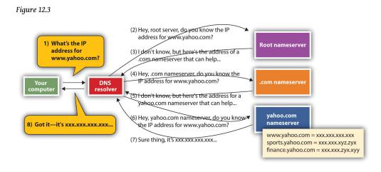
When your computer needs to find the IP address for a host or domain name, it sends a message to a DNS resolver, which looks up the IP address starting at the root nameserver. Once the lookup has taken place, that IP address can be saved in a holding space called a cache, to speed future lookups.
