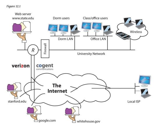
The Internet is a network of networks, and these networks are connected together. In the diagram above, the "state.edu" campus network is connected to other networks of the Internet via two ISPs: Cogent and Verizon.
