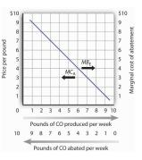
A car emits an average of 10 pounds of CO per week when no restrictions are imposed—when the price of emissions is zero. The marginal cost of abatement  $(MC_A)$  is the cost of eliminating a unit of emissions; this is the interpretation of the curve when read from right to left. The same curve can be read from left to emitting them would be very high. As more of a pollutant is emitted, however, its marginal benefit falls—the cost of preventing these units of pollution becomes quite low.
