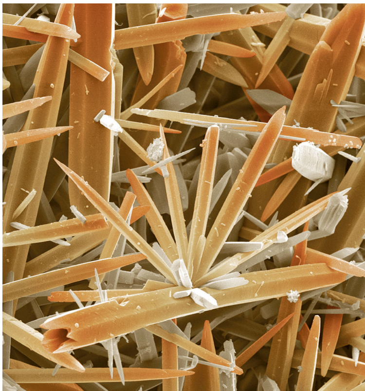
Scanning electron micrograph of kettle scale. Hard water is a solution that consists largely of calcium and magnesium carbonate in \text{CO}_2 -rich water. When the water is heated, \text{CO}_2 gas is released, and the carbonate salts precipitate from solution and produce a solid called scale.
