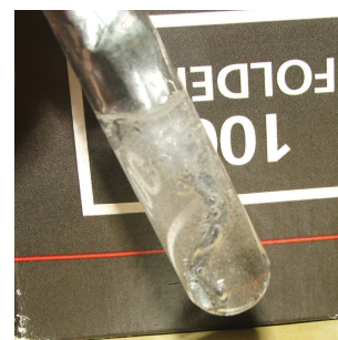
Figure 5.4 Zinc Metal plus Hydrochloric Acid
