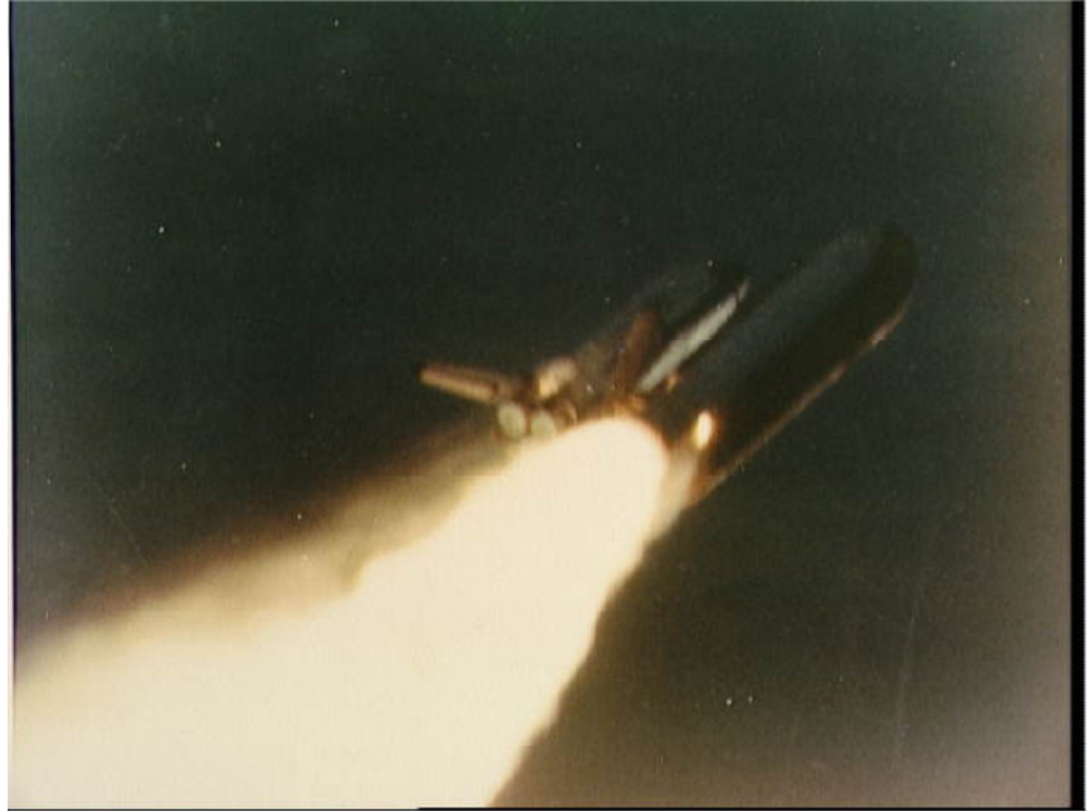
Frozen O-ring fails to seal-fire burns through. Image reprinted from NASA Johnson Space Center.
